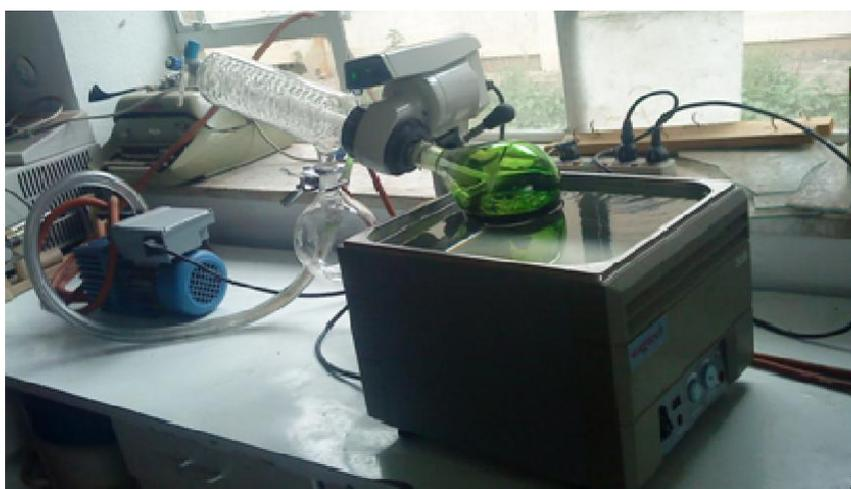
**Figure 2.** MeOH extract concentration using rotary evaporator
