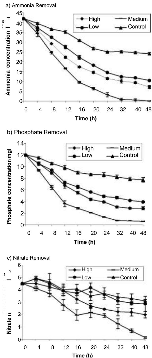
**Figure 1.** Residual concentrations of: a) ammonia, b) phosphate and c) nitrate in wastewater during the experimental period in different bioreactors. (High =  $3 \times 10^6$  cells bead<sup>-1</sup>; Medium =  $1.5 \times 10^6$  cells bead<sup>-1</sup>; Low =  $3 \times 10^5$  cells bead<sup>-1</sup> and Control = blank beads).
