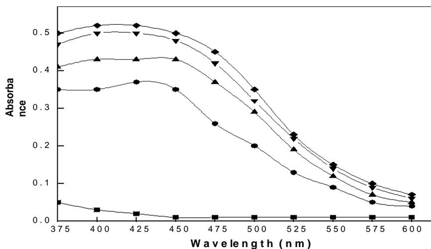
**Figure 5.** Absorption spectra of extract (■) and its reaction product with  $[Ag^+] (= 16.0 \times 10^{-4} \text{ mol dm}^{-3})$  as a function of time. *Reaction conditions:*  $[CTAB] = 4.0$  (A) and  $8.0 \times 10^{-4} \text{ mol dm}^{-3}$  (B);  $[extract] = 5.0 \text{ cm}^3$ , Time = 5 (●), 10 (▲), 20 (▼) and 30 min (◆).
