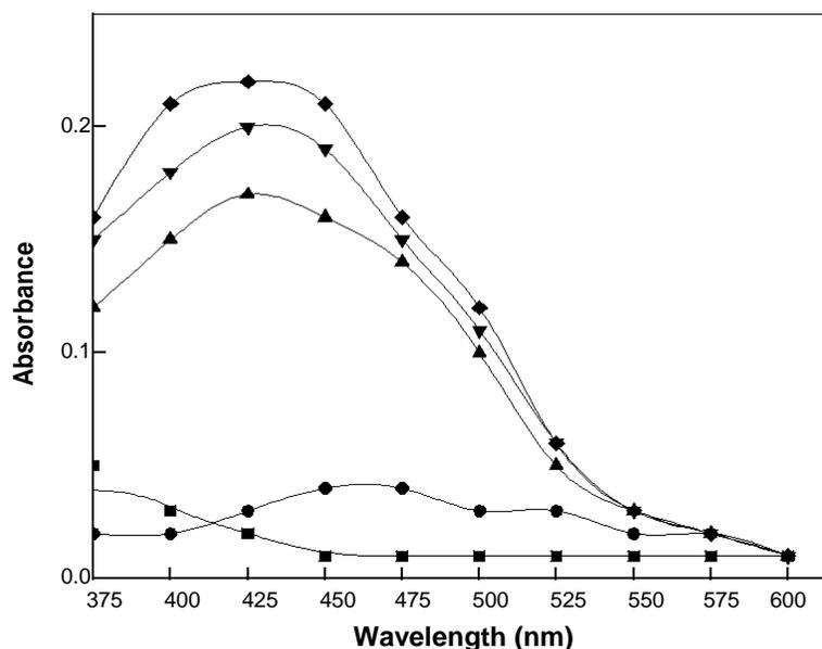
**Figure 3.** UV-vis bioreduction kinetics of the reaction of *Oriental plane* leaves extract with aqueous  $\text{AgNO}_3$  with different time intervals. Reaction conditions:  $[\text{Ag}^+] = 16.0 \times 10^{-4} \text{ mol dm}^{-3}$ ,  $[\text{extract}] = 1.0 \text{ cm}^3$ ; (■), Time = 5 (●), 10 (▲), 20 (▼) and 30 min (◆).
