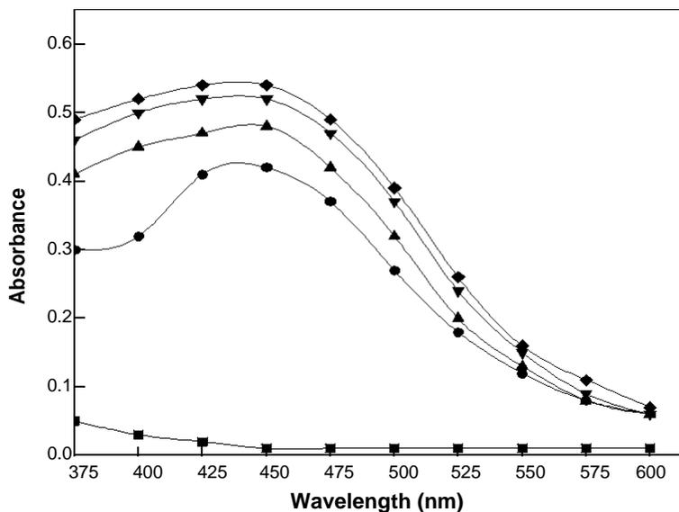
**Figure 2.** UV-vis bioreduction kinetics of the reaction of *Oriental plane* leaves extract with aqueous  $\text{AgNO}_3$  with different time intervals. Reaction conditions:  $[\text{Ag}^+] = 16.0 \times 10^{-4}$ ,  $[\text{extract}] = 5.0 \text{ cm}^3$ ; (■), Time = 5 (●), 10 (▲), 20 (▼) and 30 min (◆).
