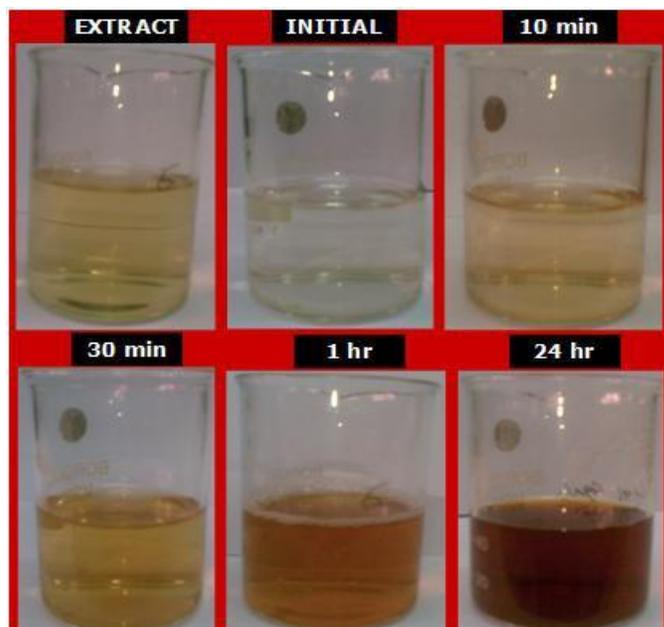
**Figure 1.** Optical images of chinnar leaves extract and its reaction product with  $\text{AgNO}_3$  at different time intervals. Reaction conditions:  $[\text{Ag}^+] = 16.0 \times 10^{-4} \text{ mol dm}^{-3}$ ,  $[\text{extract}] = 5.0 \text{ cm}^3$ , Temperature =  $30^\circ \text{C}$ .
