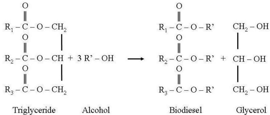
**Figure 3.** Schematic representation of the transesterification reaction.
