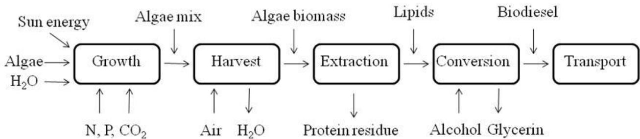
**Figure 4.** Integrated system to the production of biodiesel from microalgae.
