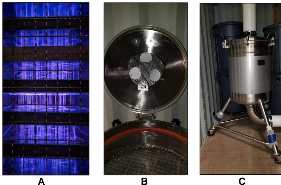
**Figure 1.** **a)** Cold plasma generator where ionization of working gas (air) occurred, producing RGS (close-up view while operating); **b)** AFB1-contaminated filter paper discs clamped in place in contacting (treatment) chamber; **c)** Sealed contacting chamber during RGS-treatment.
