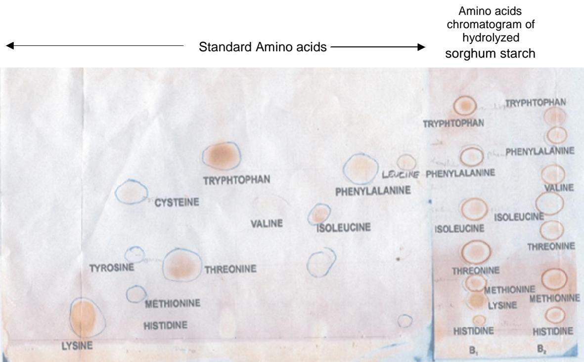
**Figure 3.** Amino acid chromatogram of hydrolyzed sorghum starch.
