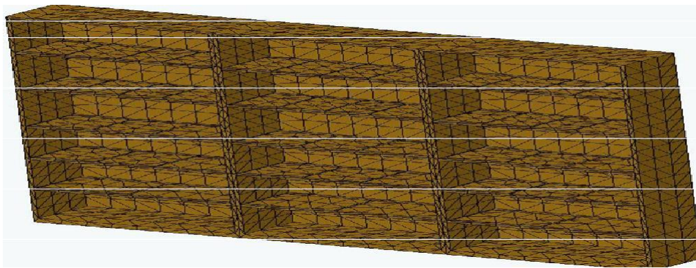
Figure 10. The mesh structure arising in finite element analysis of the bookcase.
