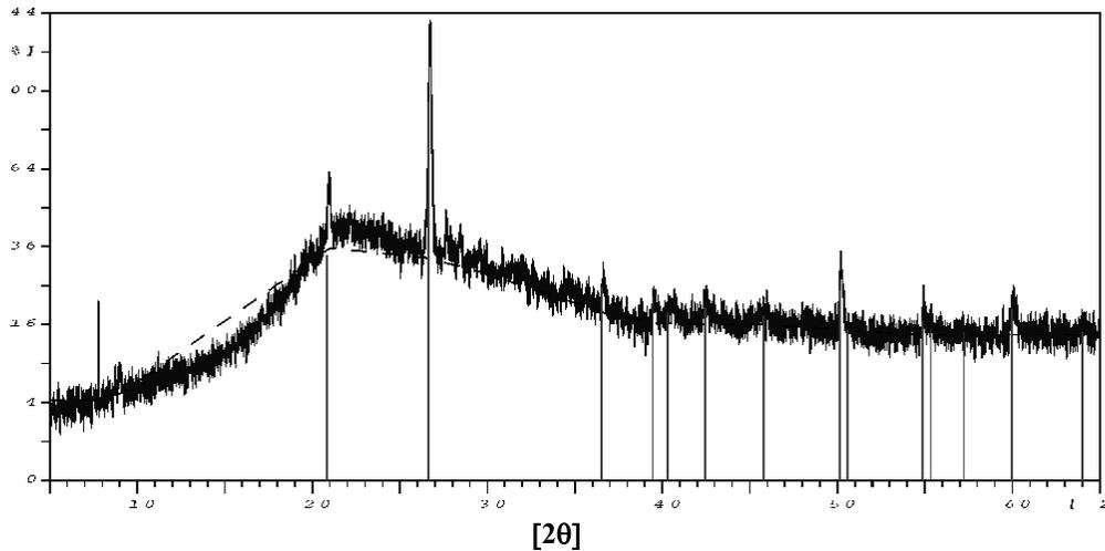
Figure 3. X-ray diffraction pattern of Bamboo leaf ash.
