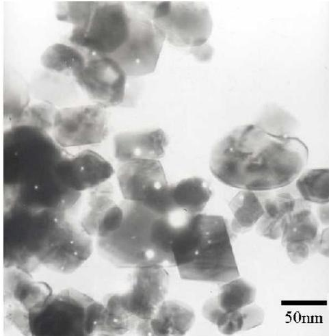
**Figure 3.** TEM images of the  $\text{Co}_3\text{O}_4/\text{CuO}$  nanopowders after calcination at  $700^\circ\text{C}$  in air for 2 h.
