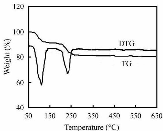
**Figure 2.** TG-DTG curves of the precursor.
