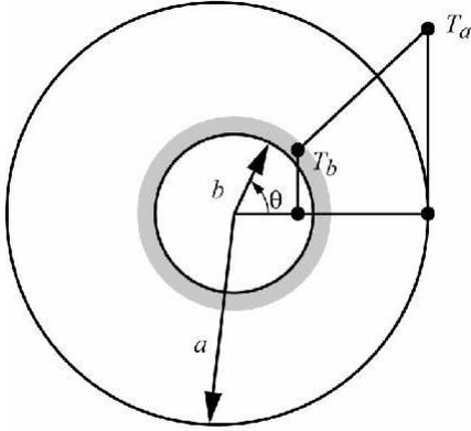
**Figure 1.** Annular plate subjected to linear temperature distribution.
