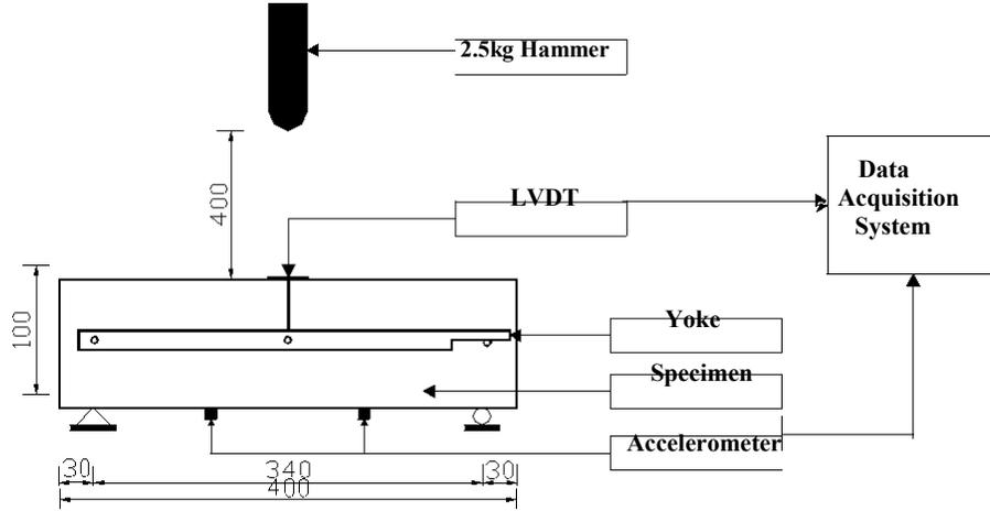
Figure 2. Drop weight flexural impact equipment.
