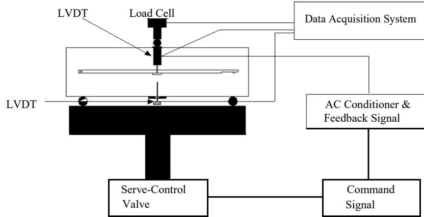
Figure 3. Schematics of flexural test setup.
