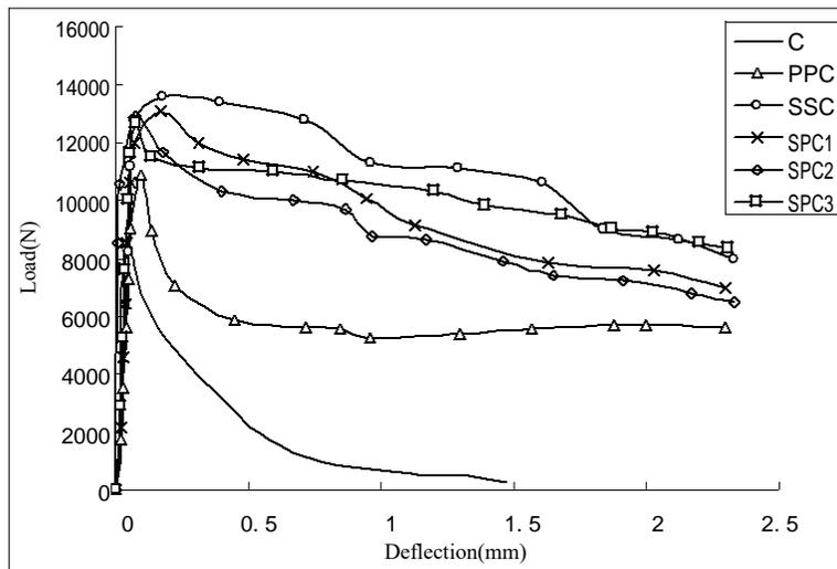
**Figure 4.** Load-deflection curves in flexural toughness tests.
