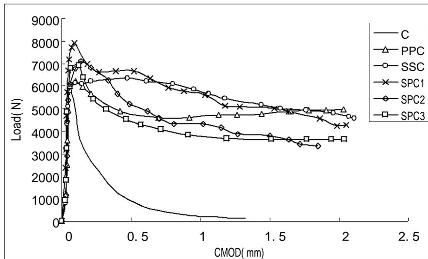
**Figure 6.** Load-CMOD curves in fracture tests.
