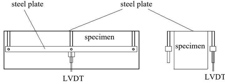
Figure 1. Flexural toughness test.
