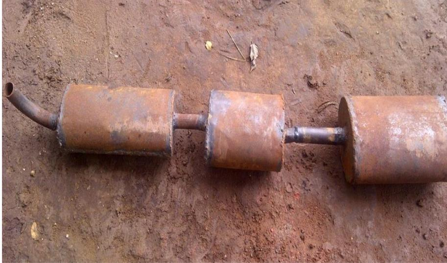
**Figure 2a.** Fabricated exhaust system.
