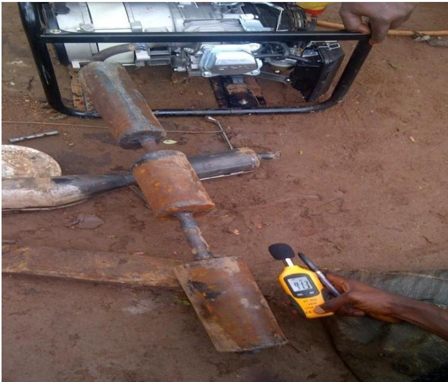
**Figure 2b.** Testing of the fabricated exhausts system attached to a generator set.
