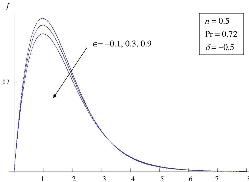
Fig. 5: The velocity profiles  $f'(\eta)$  for various values of  $\epsilon$  at  $n = 0.5, \delta = -0.5$  and  $Pr = 0.72$ .
