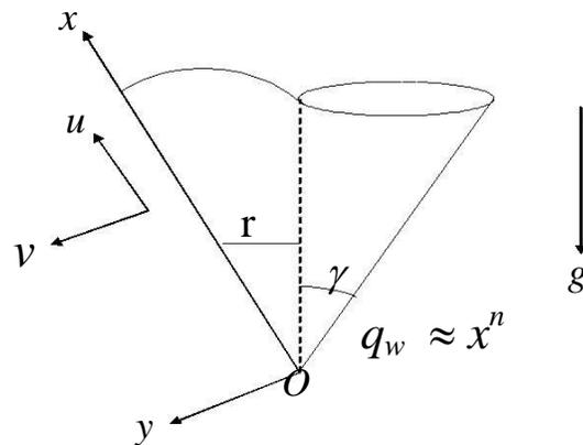
**Fig 1: Physical model and coordinates system**
