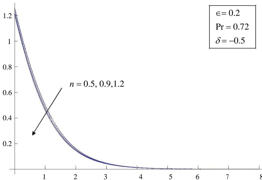
Fig. 6: The temperature profiles  $\theta(\eta)$  for various values of  $n$  at  $\epsilon = 0.2, \delta = -0.5$  and  $Pr = 0.72$ .
