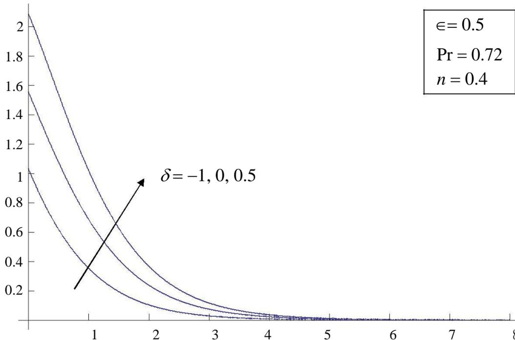
Fig. 8: The temperature profiles  $\theta(\eta)$  for various values of  $\delta$  at  $\epsilon = 0.5, n = 0.4$  and  $Pr = 0.72$ .
