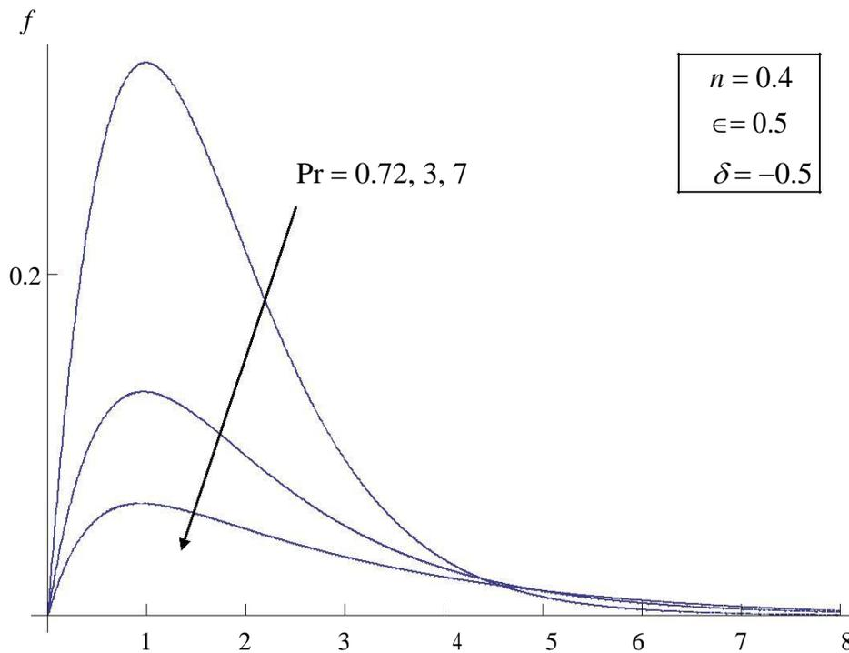
Fig. 3: The velocity profiles  $f'(\eta)$  for various values of  $Pr$  at  $n = 0.4, \delta = -0.5$  and  $\epsilon = 0.5$ .
