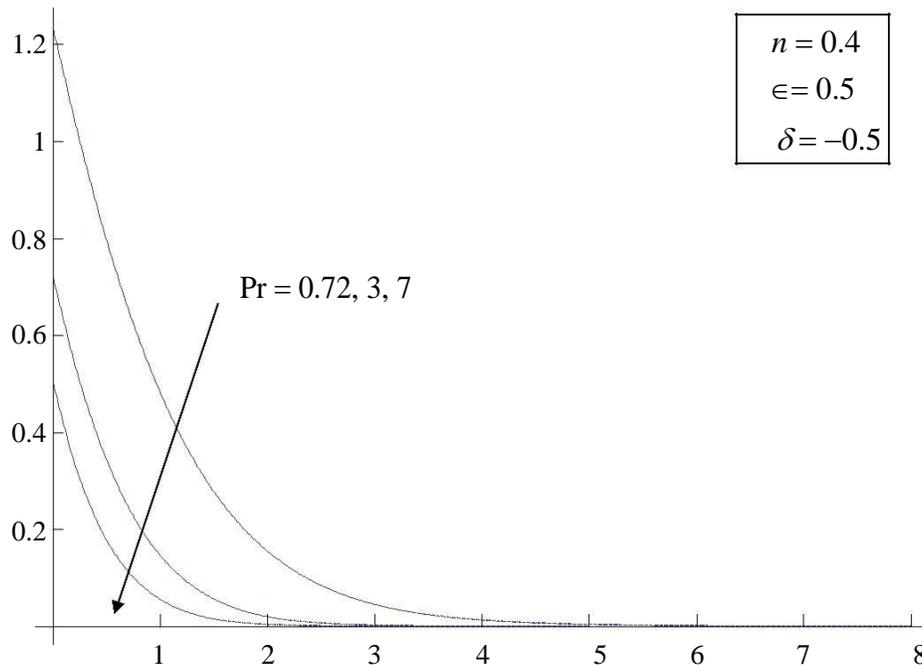
Fig. 2: The temperature profiles  $\theta(\eta)$  for various values of  $Pr$  at  $n = 0.4, \delta = -0.5$  and  $\epsilon = 0.5$ .
