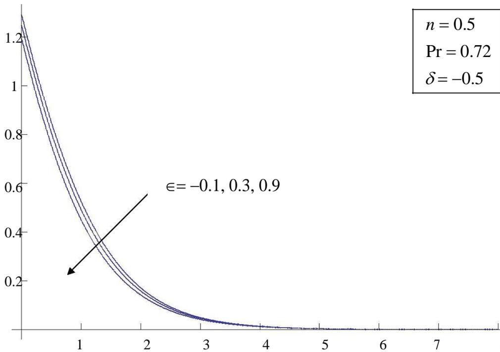
Fig. 4: The temperature profiles  $\theta(\eta)$  for various values of  $\epsilon$  at  $n=0.5, \delta=-0.5$  and  $Pr=0.72$ .
