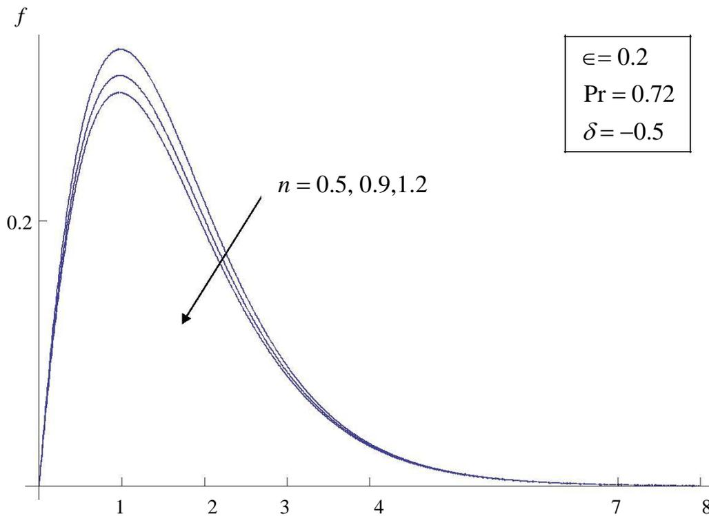
Fig. 7: The velocity profiles  $f'(\eta)$  for various values of  $n$  at  $\epsilon = 0.2, \delta = -0.5$  and  $Pr = 0.72$ .
