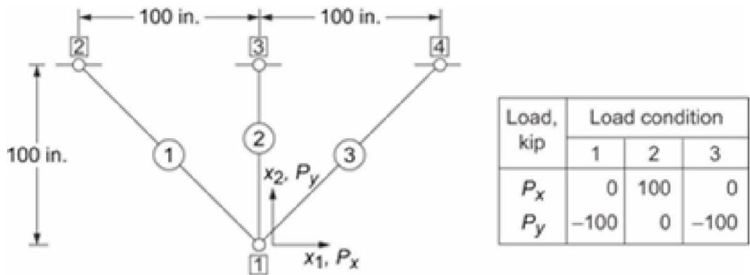
Figure 2. Three-bar truss.
