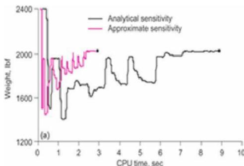
**Figure 8.** CPU solution time for SQP algorithm-twenty-bay truss.
