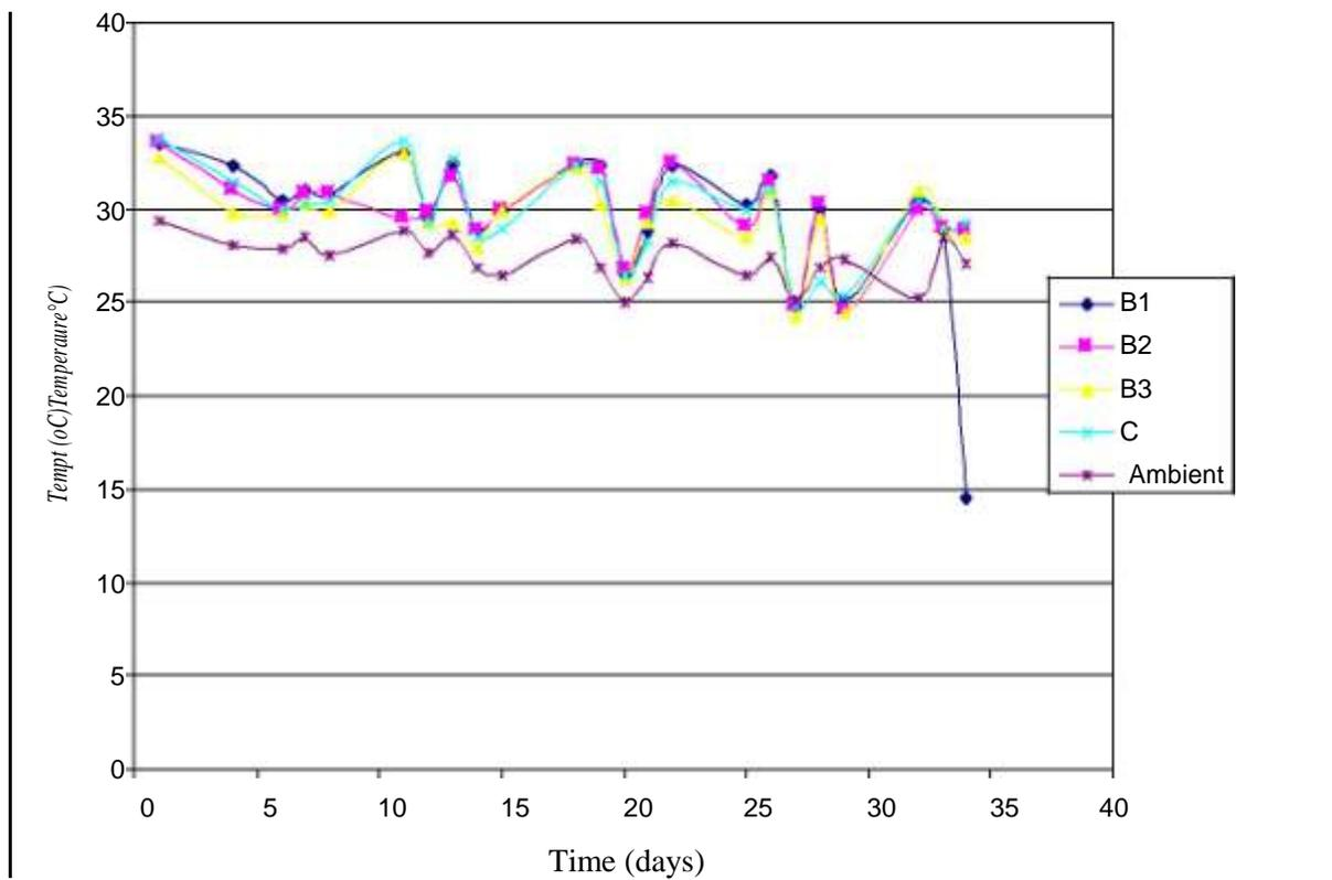
Figure 3. Average slurry and ambient temperature variation.
