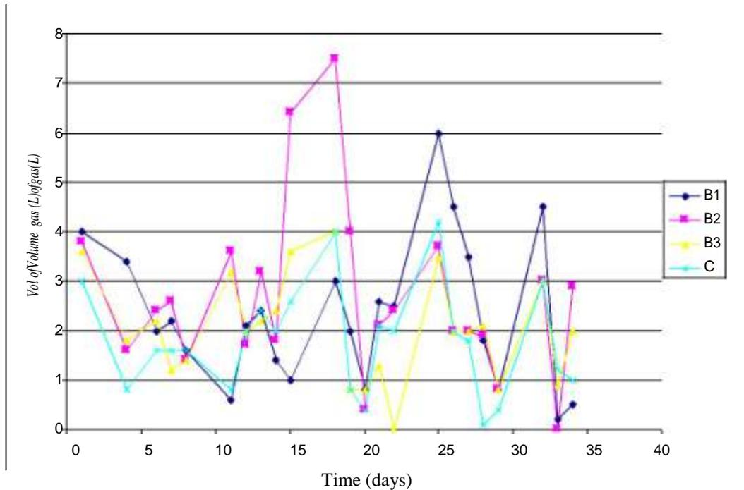
**Figure 1.** Daily biogas production pattern in the wastes.
