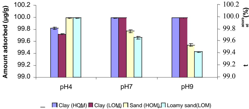
Figure 3. Effect of pH on adsorption of salinomycin at 100 µg/g soil.
