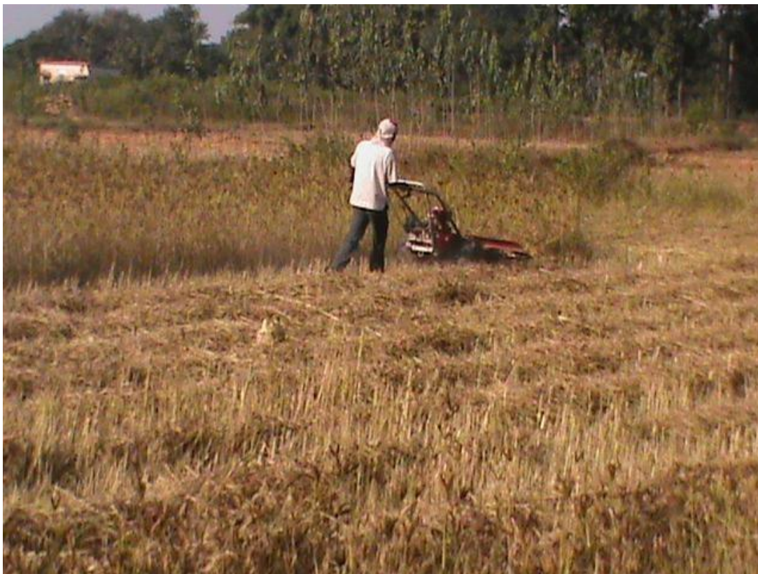
Figure 10. Harvesting of finger millet by reaper at farmer' field.
