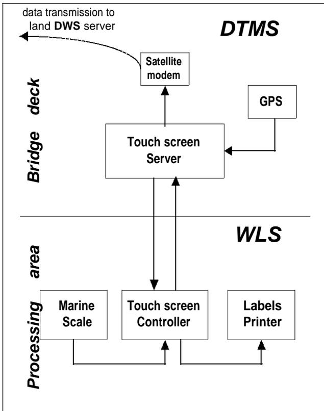
**Figure 1.** The fishing vessel operations and data flow. Video of the system is available: [http://lnx.utp-iamc.org/index.php?option=com\\_content&task=view&id=22&Itemid=29](http://lnx.utp-iamc.org/index.php?option=com_content&task=view&id=22&Itemid=29).
